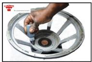
Step 4: Apply a bead of glue (black) to basket where spider and cone edge will fit.
