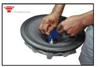
Step 6: Insert plastic shimm through the air gap between voice coil and center yoke
