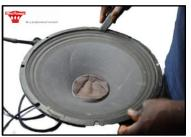
Step 1: Using utility knife, remove old cone/voice coil assembly, unsolder leads
