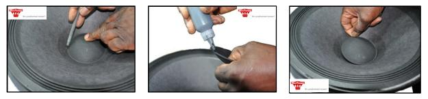
Step 9: Remove shimm, glue the dust cap in place.
